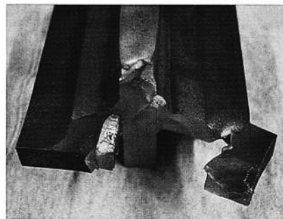
[Vertical Upward: AFR (LTTB)-8-V/U] (150 N/mm 2 , 2.66 × 10 6 cycles)
