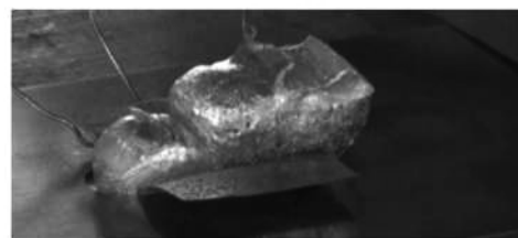
(c) Foaming of porous A6061
