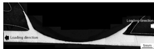
Fig.7 Cross-sectional OM image of the specimen after the tensile shear strength test (Pd:1.8mm).
