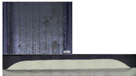
Wide, flat cladding layer which was provided by beam control
