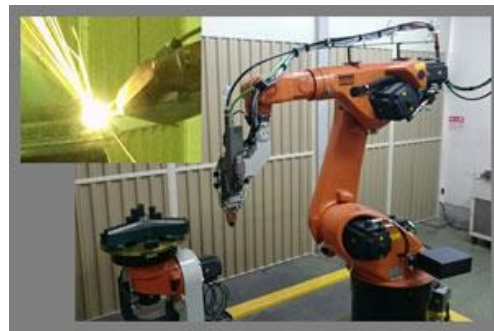
Experimental apparatus for laser cladding
